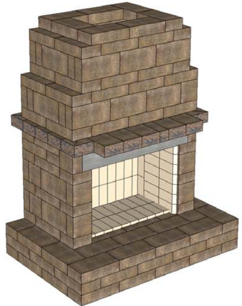
16. Stack next course with side inset. See 14.
