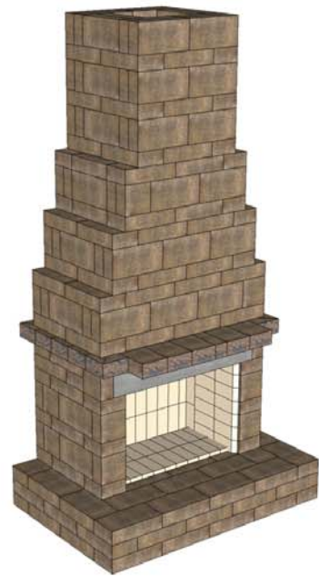
20. Stack chimney to desired height.
