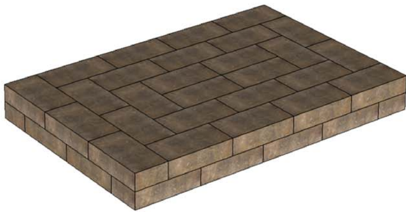
02. Second course should be reverse of 1st course so that joints do not line up. This will stabilize base.
