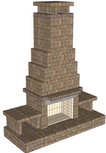
28. Set wood box tops as shown. Glue blocks together in pairs (short ends) day before. Stand up to let dry. Weight will help secure bond.
